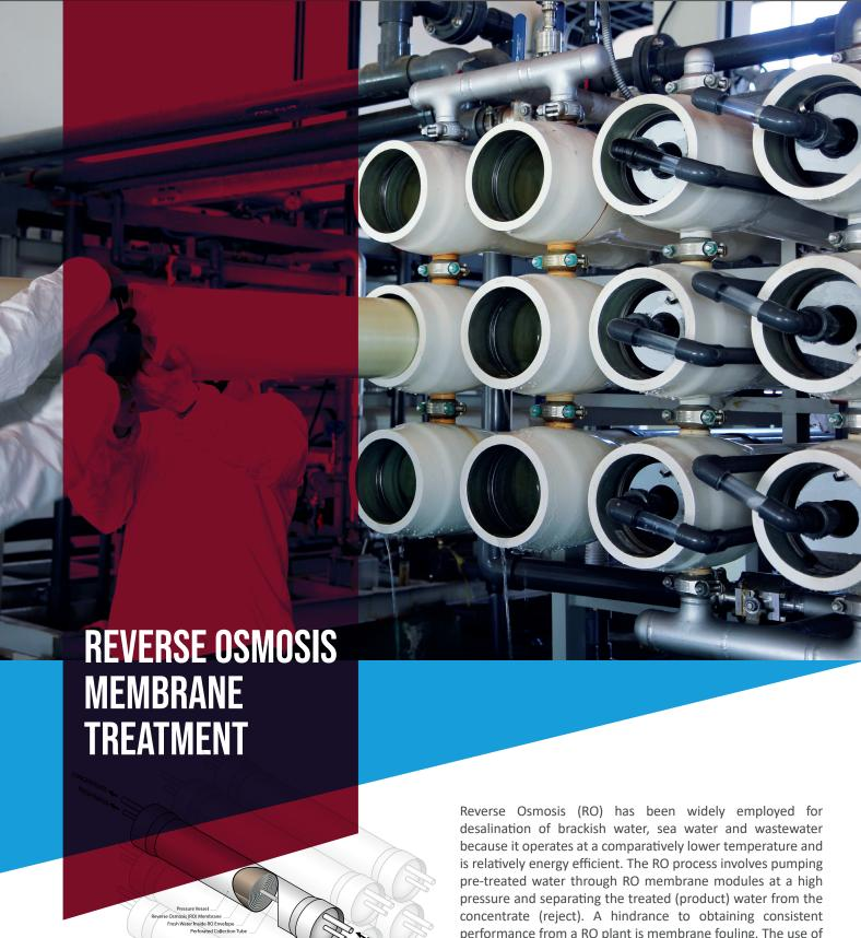
performance from a RO plant is membrane fouling. The use of antiscalants, preservatives, cleaners, and fouling control products are known to provide total membrane protection and prolong their productive life. Chembond Water Technologies offers the entire range of proven RO membrane treatment products to minimize losses arising from fouling.
